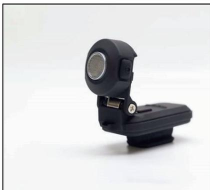
The BuzzClip is a small and discreet wearable device for people living with blindness or partial sight. The device uses ultrasound to detect obstacles that are in one's path. It notifies the user of these obstacles through intuitive vibrations, allowing the user to safely navigate around objects that they may encounter. The BuzzClip offers essential head level obstacle detection and can be easily held or attached to most clothing, making it a highly versatile and useful device.
